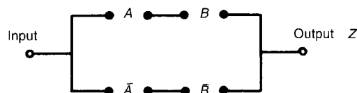
(b) Switching circuit for Z = A \cdot B + \bar{A} \cdot \bar{B}
